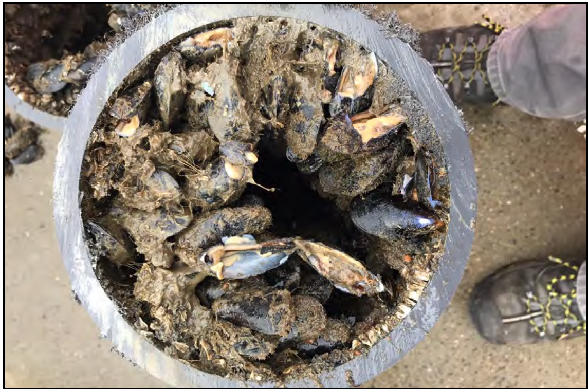
Photo 4: Example of biofouling that can occur within intake pipes
